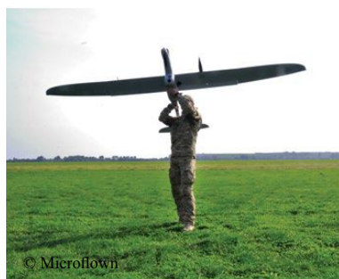
Figure 4 Acoustic Pointer Integrated on Hand-launched UAV
